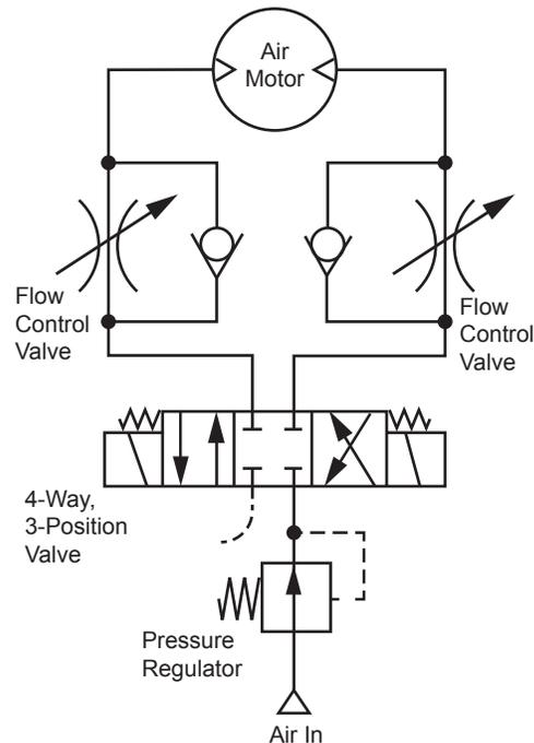
**Figure 8.** Torque and speed control of a reversible air motor.
