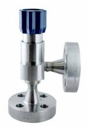
The BP-MF690 is a back pressure regulator for gas or liquid applications suited for typical low flow applications to xxlpm (liquid). The liquid version includes ceramic seating for ultimate protection against cavitation and erosion on aggressive application media such as water glycol and methanol. This accurate regulator controls inlet pressure and vents excess pressure back via the threaded ¾" NPT outlet port.
