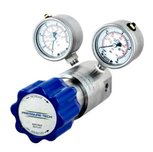
Designed with precision machined sensing elements to allow fine pressure control on pressures up to 414bar. Two piston sensors combined with two spring ranges, provide 4 outlet control options with a combination of low torque adjustment and excellent sensitivity. A self venting design and optional ratio loaded actuator makes it an ideal regulator for use with electro-pneumatic controllers for automated pressure control.
