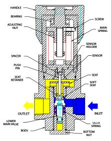
\*Assembly drawing for reference only. Refer to office for specific detail
